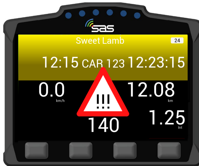
SCREEN 11. HAZARD proximity warning
