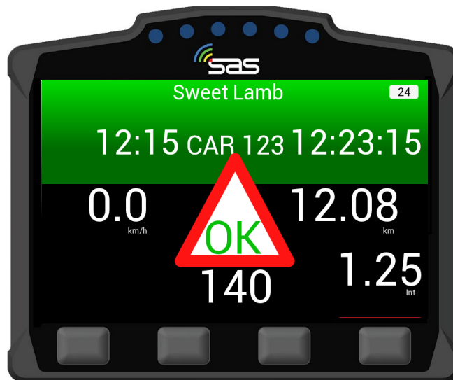
SCREEN 10. OK proximity warning
